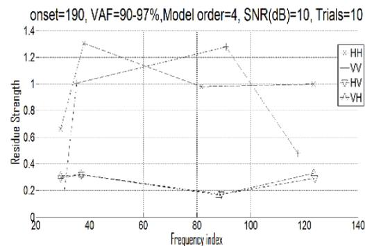
Fig 4. The quadrature-polarized residue pattern with the early time excluded.
