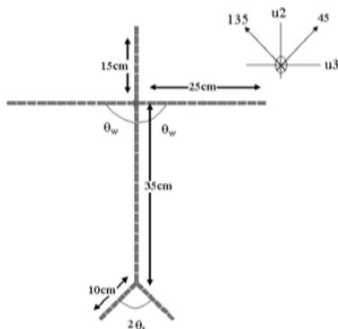
Fig.1. Dimensions (in cm) of the generalized aircraft model. The angles  $\theta_w$  and  $\theta_t$  give the model different shapes, but do not change the model dimensions.
